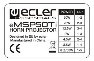
Figure 1: rear panel's power selector
