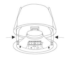
**Step 4:** follow step D. Then connect the audio cable to the loudspeaker's terminal block. Finally, insert the mounting springs into the hooks and push the loudspeaker into the back can.
