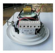
**Step D:** connect the loudspeaker wire according to the requirement in the label. Then install the loudspeaker.
