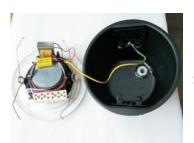
**Step B:** release the spring to open the fireproof dome.
