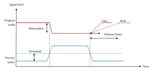
The priority mode allows adjusting the attenuated signal recovery time (PRIO RELEASE TIME), by means of a switch FAST / SLOW located at the rear panel.
