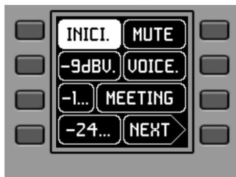
Pressing the same key a second time performs the selection action, showing in negative the new option (preset), already active (= preset activated):
