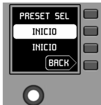
In this menu, S3 displays the active preset, while S2 flashes the options of the assigned carousel of available presets as you navigate through the K5 turn:
