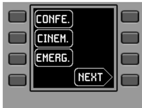
The long press (> 5 seconds) of any key, K1 to K8, shows the configuration parameters of the unit: name, model, firmware version and Ethernet network connection parameters:
