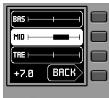
Changes to these settings are in real time and do not require K5 to be pressed or any other action to confirm. However, a long press of K5 (>3 seconds) within this menu resets the EQ filters to 0 (flat equalization).
