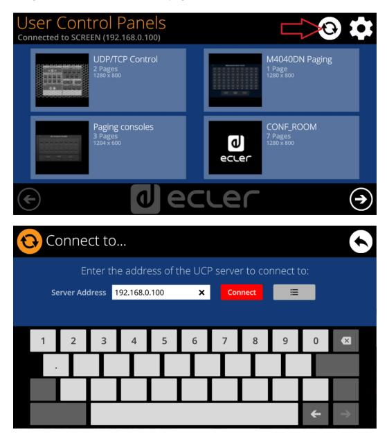
This page allows deciding the UCP server the unit will connect to as a client. The UCP server may be a computer, a MIMO4040DN matrix (yes, it has an embedded UCP server in its engine!) another WPNETTOUCH / WPmSCREEN unit or even the same WPNETTOUCH unit. In any case, the UCP server shall host and run an EclerNet Manager project that includes a series of UCPs which can be remotely managed by any UCP client.
