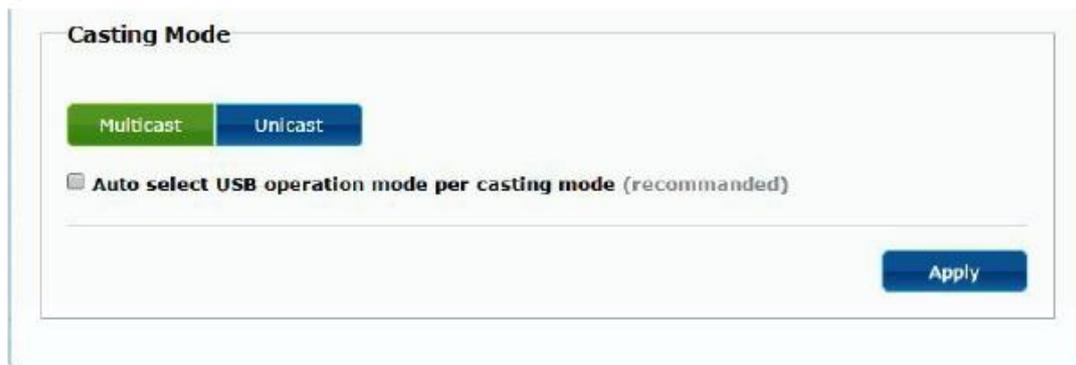
The "Auto select USB operation mode per casting mode" allows you to change the behaviour of the USB pass-through according to the selected casting mode.
