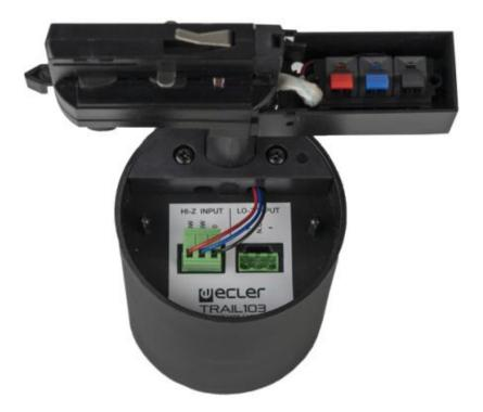
To make the connection in the speaker, it has a male Euroblock type connector, which is connected to the high or low impedance input (**HI-Z IN** or **LO-Z IN**), depending on the type of installation:
