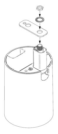
**4.** Make the connections, taking into account the colour coding for high and low impedance explained in point 3 of the instructions for installation on the lighting rail. If desired, use the screwable rail on the base of the surface mount. Attach the speaker to the threaded bar or truss and orient the speaker to the desired position along the vertical and horizontal axes
