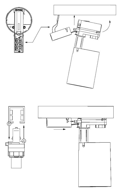
Connection to a rail GLOBAL Trac Pro (three-wire lighting anchorage system)
