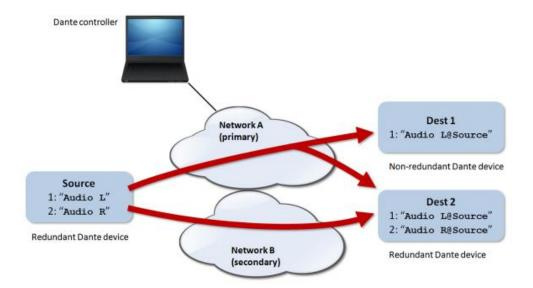
**Note:** in this mode, if (by mistake) the primary and secondary ports connect to the same Ethernet network, Dante Controller will no longer have access to the network configuration control and routing DANTE<sup>TM</sup>/AES67 of the MIMO4040CDN ports. This control is recovered when one of them is disconnected from the same network as the other.
