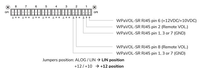
WPaVOL-SR connection to MIMO serial GPI ports
