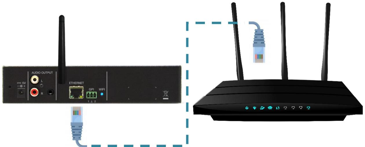
Figure 14 : example of connection via the Ethernet network interface (cable)
