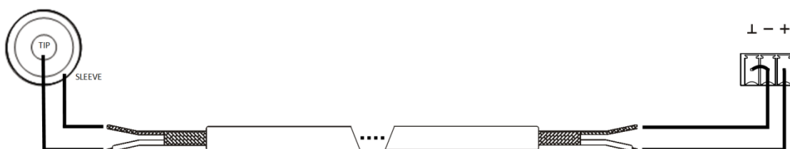
4. Connection of unbalanced output to balanced input
