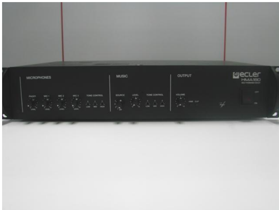
ECLER HMA 180 – Control Panel
