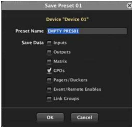
When you recall this presets using button press on the UCP panel, GPO configuration status (active/inactive) that was stored into a preset will be loaded, without changing any other device configuration.
