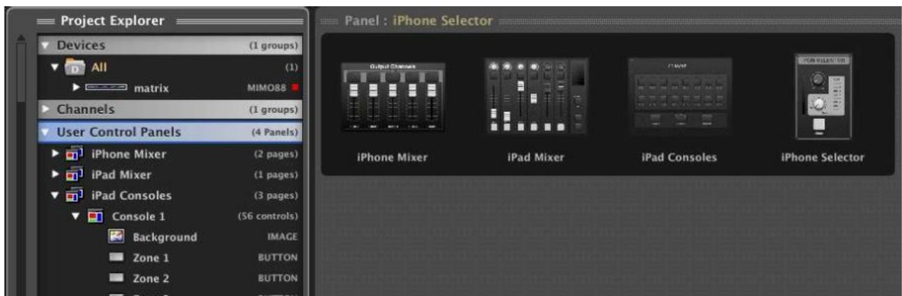
Computer which runs EclerNet Manager, which executes EclerNet project which contains project panels, is converted into web server and UCPs can be accessed and used from remote devices which function as clients. These devices can be computers, tablets, smartphones, WPNETTOUCH screen, etc.
