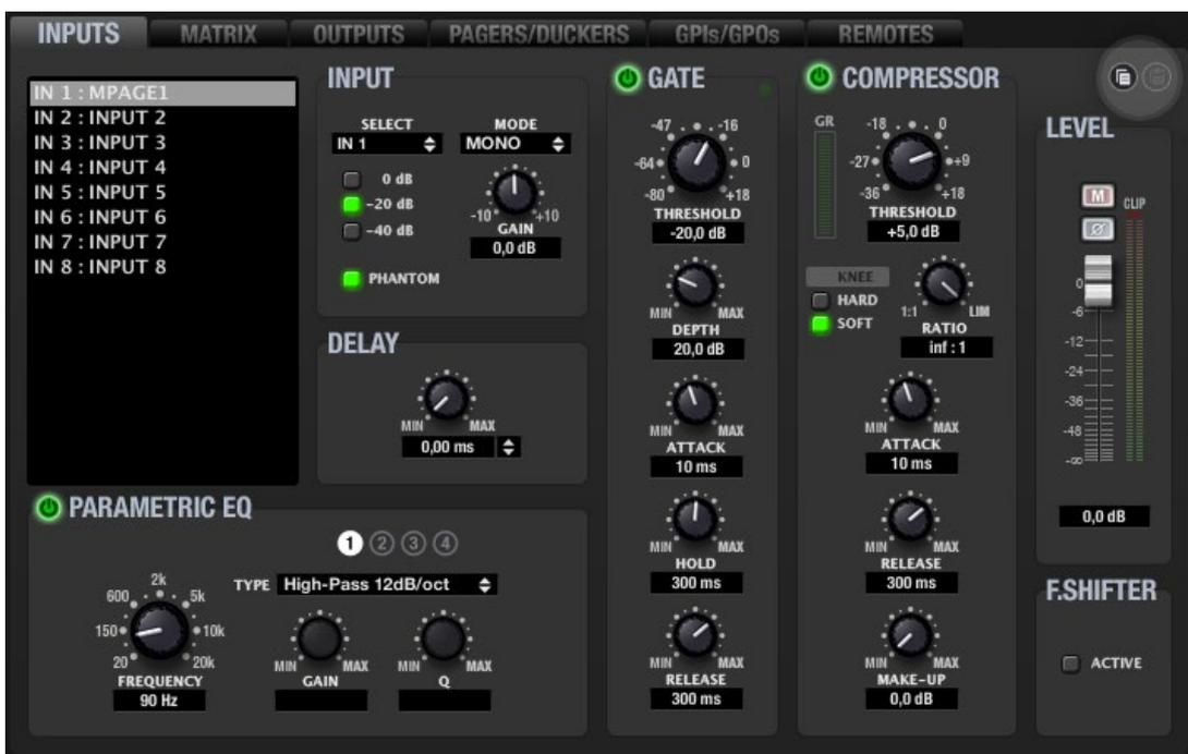
It's recommended to use high-pass filter to reduce manipulation noise. Typically between 90 and 150Hz.
