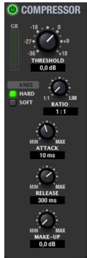
It's not simple to correctly configure delay time for ATTACK and RELEASE parameters. Using short delay time for attack and release can cause noticeable distortion and excessive in low frequencies. When using long delay time can make the compressor useless, causing it to activate too late, allowing signal peaks of elevated intensity without applying any compression.
