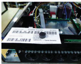
The amplifiers are barcoded for speeding up SMT assembly
