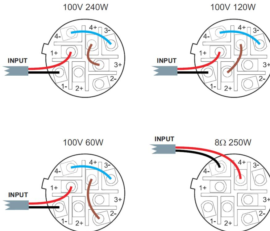
Figure 1: Speakon® connection diagram
