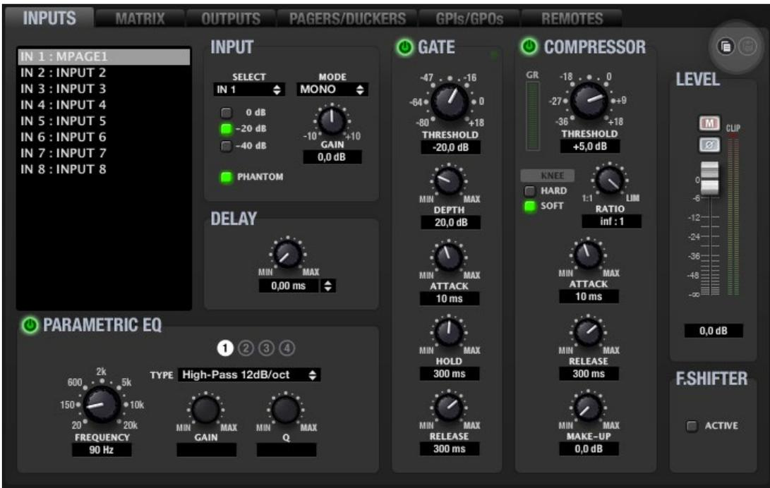
It's recommended to use a high-pass filter to reduce manipulation noise. Typically between 90-150Hz.
